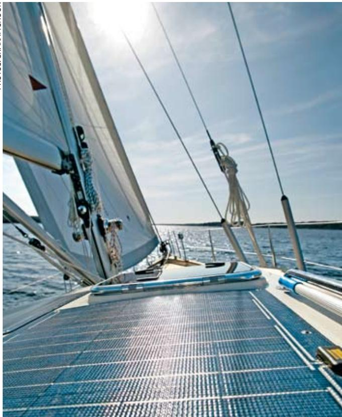
Semi-flexible panels can be mounted on deck and have a non-slip surface
