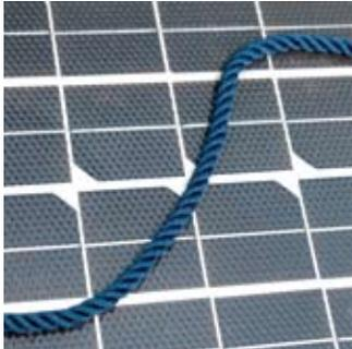
We also measured the effect of a rope laid across each panel
