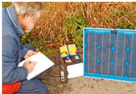
*Test in progress: Emrhys monitors a panel's performance while it tops up a marine battery*
